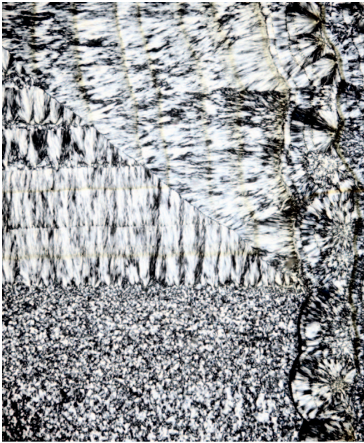
FIG. 2. Photomicrograph of a thin section from the extreme right end of the agate sample shown in Figure 1. Three types of silica polymorphs are visible: the vertical band on the right is an assemblage of small opal-CT spherulites composing the outer 3–4 mm thick brown envelope of the agate sample; the horizontal band at the bottom of the section is microgranular (20–60 μm) and partly microglobular cristobalite aggregate; the upper part is fibrous chalcedony spherulites in horizontal and vertical bands, each having a basic zone of shape-preferred orientation initial growth. Nicols are crossed. FOV 2.5 mm wide.
