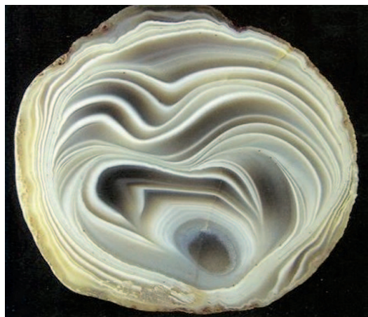
FIG. 14. Agate from Mashatu, Botswana, with concentric layers crumpled due to amygdule contraction. Sample is 6.5 cm wide. Photo and collection of Johann Zenz.
