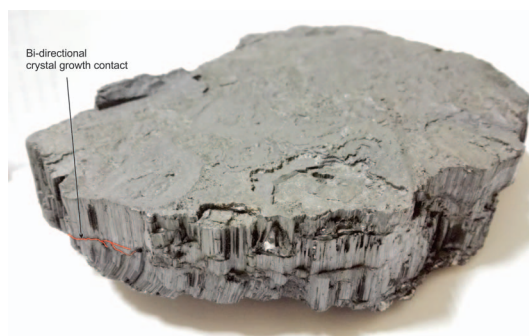
FIG. 2. Approximately 30-cm long, 6-cm thick hand sample comprising a cryptomelane-todorokite mineral assemblage exhibiting distinct acicular crystals. The crystal growth occurred perpendicular to the fracture plane in which it formed. The contact between the bi-directional crystal growth is clearly distinguishable in the center of the sample.
