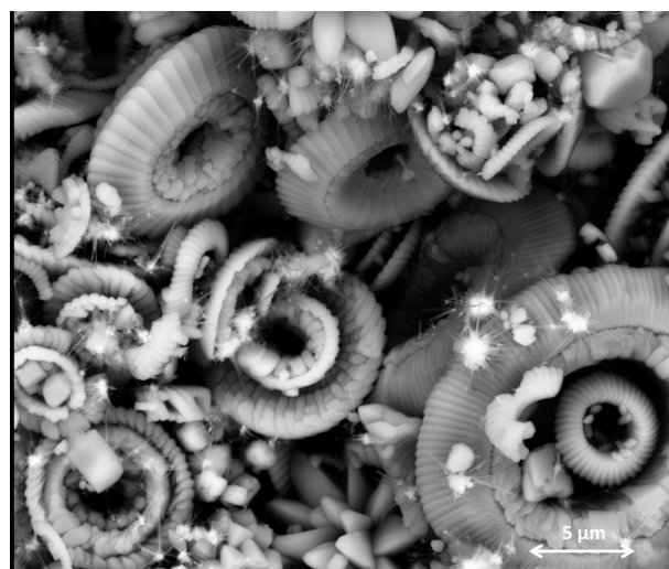
FIGURE 5. BSE SEM image of a nodule from nearby Site 1265 (sample 1265A-18H-CC, earliest Oligocene) composed primarily of calcareous nannofossils with clusters of needle-like crystals of Mn oxide, presumably todorokite.
