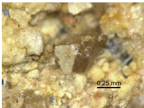
Figure 1. A photomicrograph of hydroxylbastnäsite-(Ce) from Kami-houri, Miyazaki Prefecture, Japan (NSM-M29287), showing a hexagonal short prismatic crystal with yellowish light brown color.
