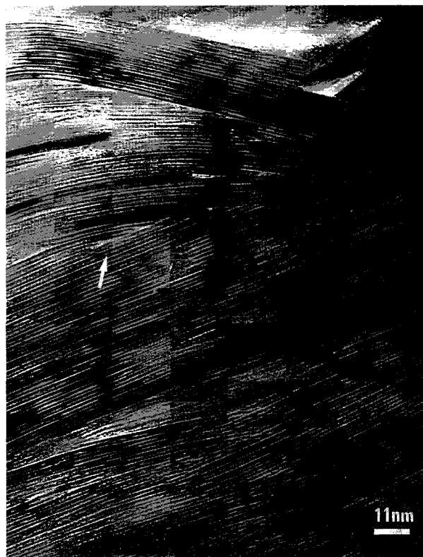
FIGURE 7. Corrensite from sample SC1603. Rosettes of corrensite crystals seen in cross section by TEM. Corrensite crystallites join as low-angle grain boundaries and edge-dislocation-like defects (white arrow). The image of the corrensite structure (e.g., upper middle and lower right) appears as a regular succession of white ~10 Å (collapsed smectite) and ~14 Å (chlorite) fringe spacings.
