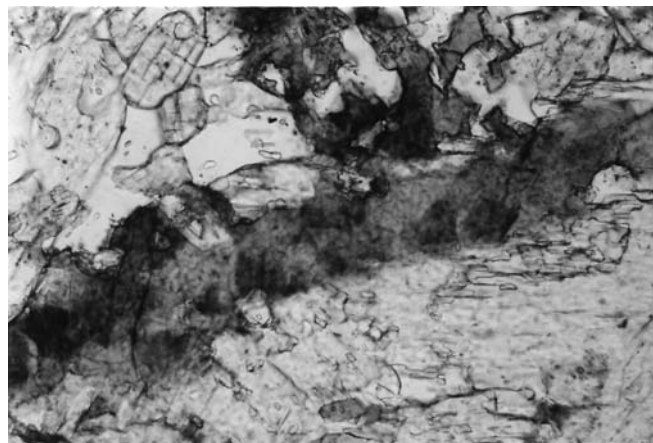
Fig. 2. Veinlet of cerchiaraites cutting a serandite-quartz aggregate in OU 68677. Replacement of serandite (light grey with cleavages) by cerchiaraites (dark) spreads from the veinlet into the upper part of the field (quartz clear). Plane-polarized light; darkest areas in the vein result from deep-green absorption tints for the e -ray; medium-dark areas result from yellow-brown colour for the o -ray. Field of view: 450 x 300 \mu\text{m} .
