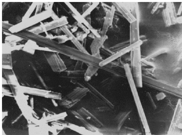
Fig. 2. SEM image of long-prismatic crystals of tashelgite. Width of image is 40 \mu\text{m} .
