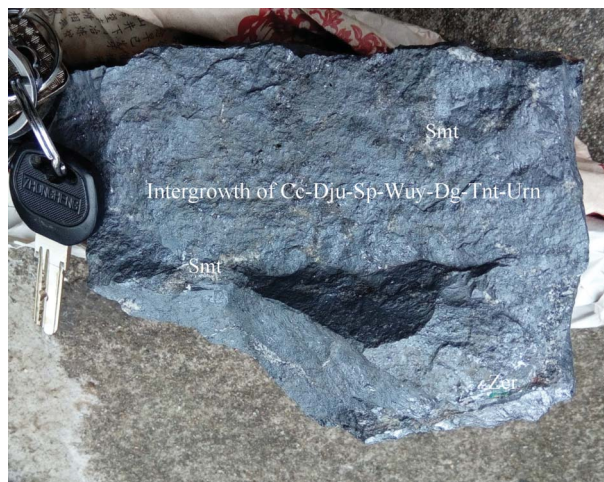
FIGURE 2. Specimen of massive chalcocite (Cc ~85%) in association with djurleite (Dju ~8%), sphalerite (Sp, ~5%), wuyanzhiite (Wuy ~1%) and minor digenite (Dg), tennantite-(Zn) (Tnt), smithsonite (Smt), pyrite (Py), uraninite (Urn), and zeunerite (Zer).
