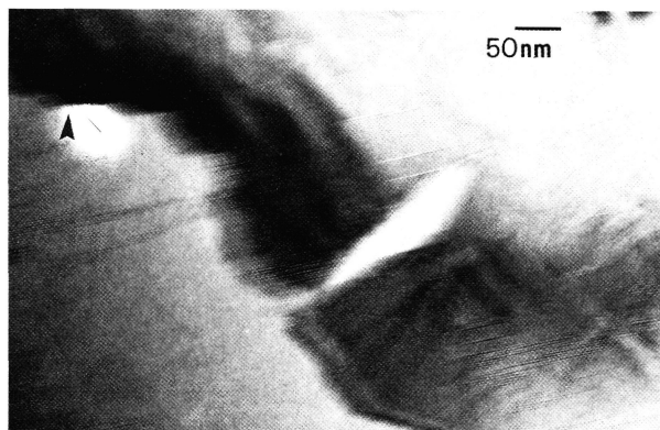
Fig. 9. Bright field image near c -axis showing fringes which are continuous across the twin boundaries (black arrow). Note the defects related to the 27\text{ \AA} repeat.
