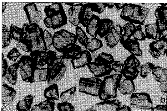
FIG. 4. Photomicrographs of apatite separates from the different rock types of the Main Mass from the NW and SW sections; sample numbers are shown in brackets. (a) Euhedral crystals of cumulus apatite from the quartz gabbro (30) on the North Range. Some of the crystals have an axial cavity (ac) parallel to the Z axis. (b) Subhedral to anhedral crystals of post-cumulus apatite from the norite (28) on the North Range. (c) Anhedral post-cumulus apatite from the norite (64) on the South Range. Note that here, all of the crystals are poorly developed and equant. Field of view for (a), (b), and (c) is 1 mm. (d) Photomicrograph (crossed nicols) of representative cumulus apatite from the quartz gabbro (30). Note the numerous cross-sections and prismatic sections. Field of view for (d) is 3 mm.
