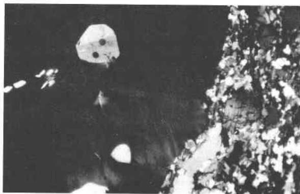
Fig. 27. Photomicrograph of schist sample W67B from the upper part of the Mount Mineral Formation, east limb of Pelham dome. To left is the margin of a high orthoclase megacryst enclosing quartz, plagioclase, and sillimanite (stout needles far left). The immediately surrounding matrix (right) contains muscovite, biotite, and coarse kyanite (large grain close to orthoclase right center).
