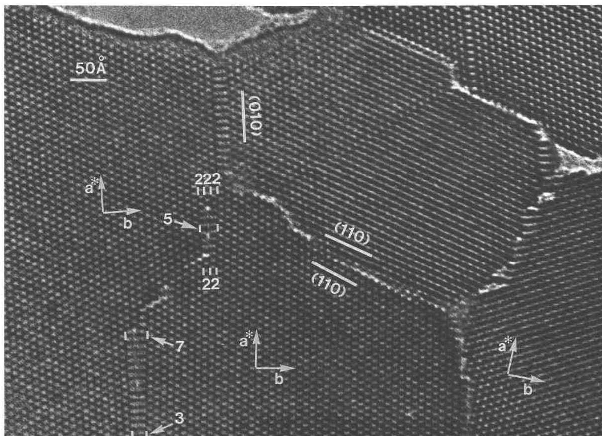
Fig. 14. A partly polygonized crystal. A small subgrain is formed by the wide chains along (010) and (110) defects. In addition, a variety of wide-chain pyriboles occur within the crystal.
