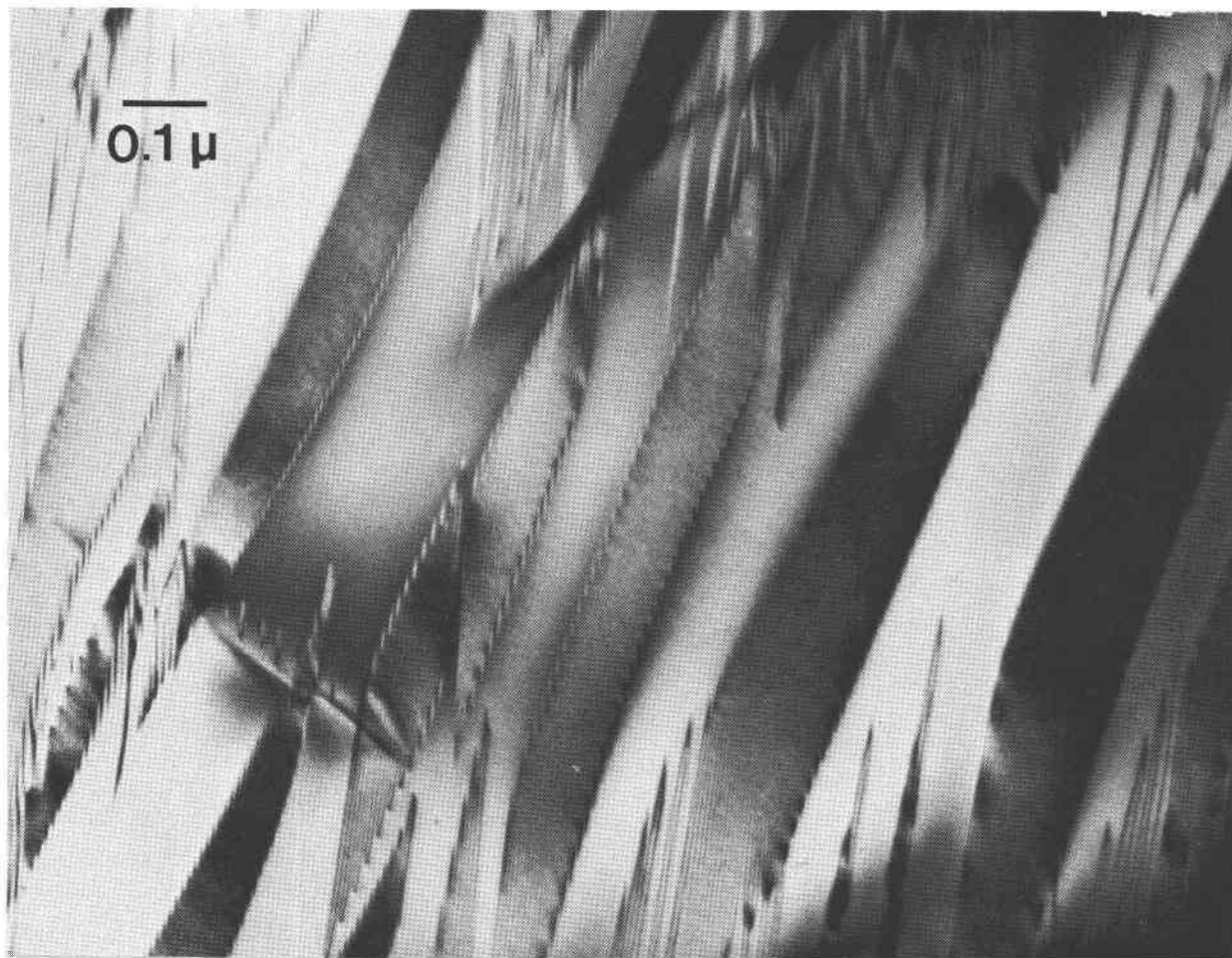
Fig. 5. Huttenlocher intergrowths in Thetford labradorite ( \sim\text{An}_{71} ). DF, g = 031 . This region was adjacent to bytownite in Fig. 3a.
